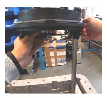
• Unscrew the screw holding in the MOBRA plunger and put the plunger, screw, and washers aside in the same order. Check kit contents 5 for plunger configuration.
