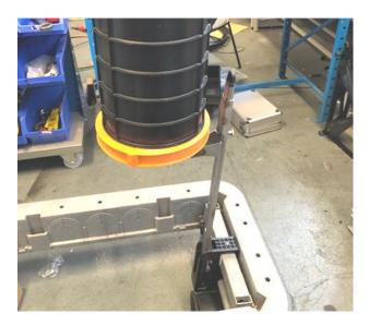
• Replace the cap and clamp and move the joint into the horizontal position.
