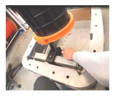
• Move the closure into the vertical position by lifting the closure and putting the black pin through the Mobra knuckle.
