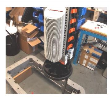
• Remove the orange clamp and cap from the LMJ to expose the internal parts of the closure.
