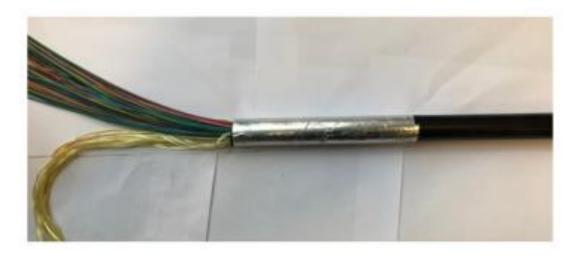
• Abrade150mm down the cable from the cable butt.
