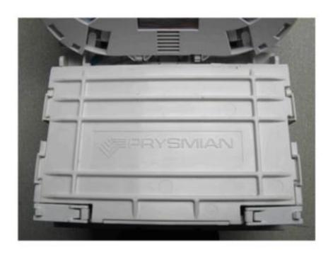
• Replace the manifold cover by clipping into place.
