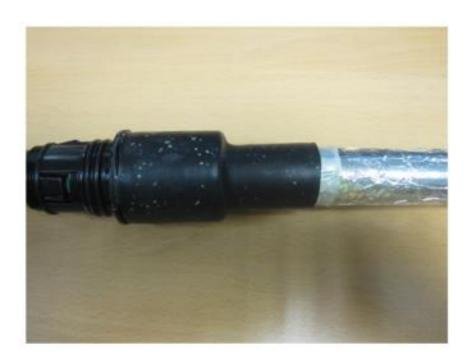
• Fully convert the heat shrink sleeve and allow cooling for 10 minutes.
