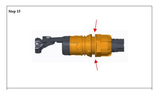
• Loosely tighten the gland nut onto the gland body assembly.
