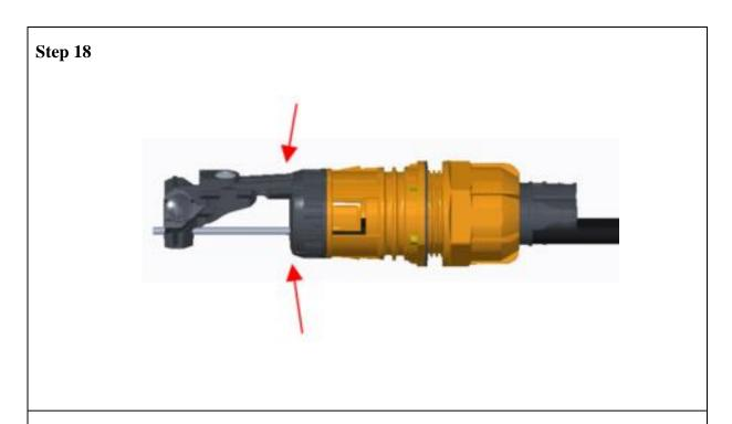
• Pull back cable so cable butt is in line with the top of the CSM clamp nut.
