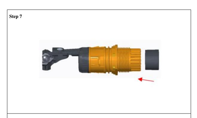
• Align the 3-way seal with the gland body assembly.
