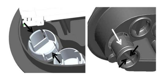
• Remove port blank from the base by fully squeezing together the tabs from inside the base.
