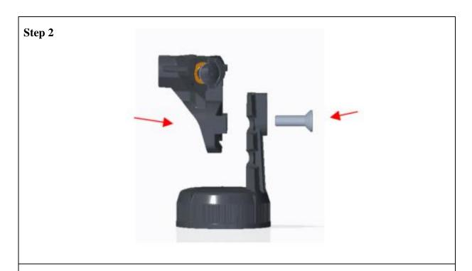
• Align the csm bracket with the 3-way CSM retention post and M4 x 12 CSK screw.
