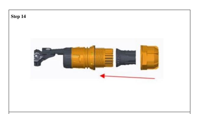
• Align the anti-torsion part and nut with the gland body assembly.
