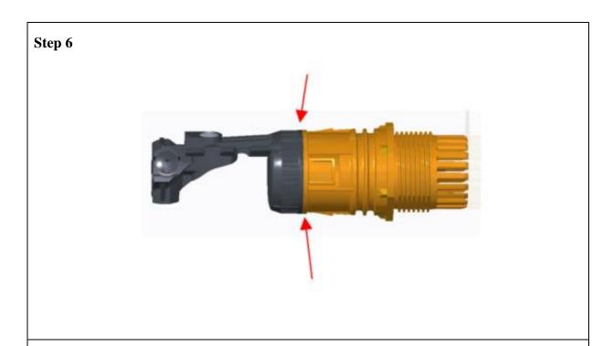
• Screw the CSM bracket into position until the faces mate.
