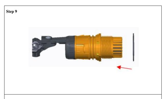
• Align the spacer with the gland body assembly.
