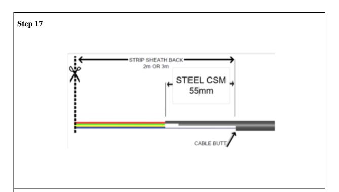
• Measure from the cable butt and cut the steel CSM to 55mm.
