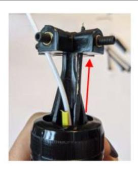
• Insert the strength member into the csm restraint hole.
