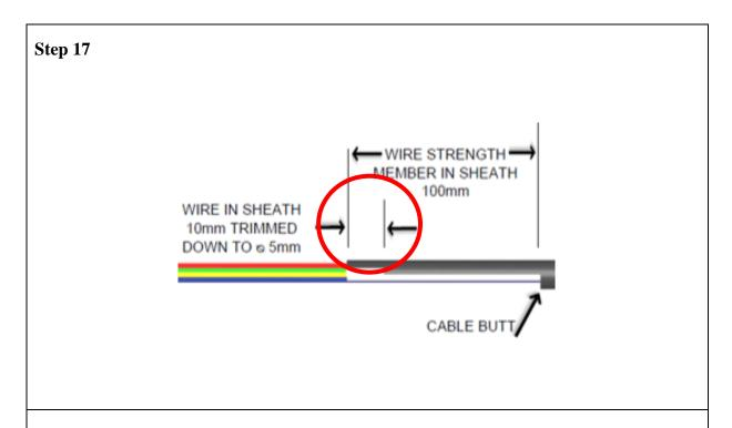
• Using an approved diagonal cutting, trim the end of the remaining sheath to a diameter of approximately 5mm such that 10mm length.
