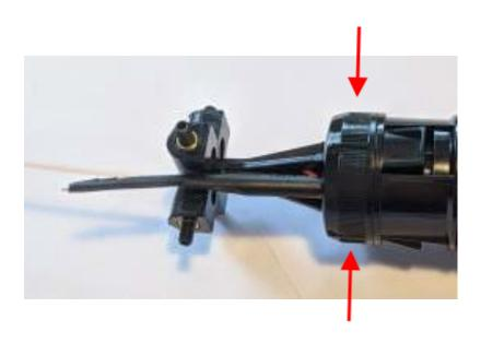
• Pull back cable so cable butt is in line with the top of the csm clamp nut.
