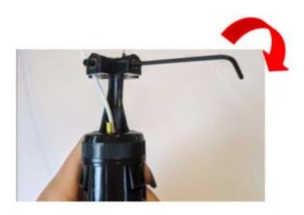
• Using a 2mm Allen key tighten the grub screw onto the strength member. Ensure the wire in the sheath strength member is caught beneath the grub screw securely or repeat this step.
