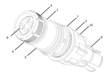
THE MECHANICAL GAS BLOCK GLAND SYSTEM IS DESIGNED FOR USE WITH HYBRID CABLE. THE SYSTEM IS USED TO BLOCK GAS AND WATER FROM LEAKING FROM THE CABLE BUTT INTO CABINETS IN THE EVENT OF CABLE SHEATH DAMAGE.
