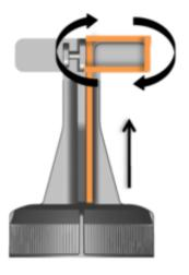
WHILST KEEPING TENSION ON THE CABLE, BEGIN TO WRAP THE ARAMID AROUND THE ARAMID CHANNEL STARTING FROM THE INSIDE TO OUTSIDE UNTIL A MINIMUM OF 1.5 TO 2 TURNS HAVE BEEN MADE.
