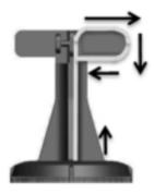
WHILST KEEPING TENSION ON THE CABLE, BEGIN TO WRAP THE STEEL/ARAMID AROUND THE CHANNEL STARTING FROM INSIDE TO OUTSIDE UNTIL A MINIMUM OF 1.5 TO 2 TURNS HAVE BEEN MADE.
