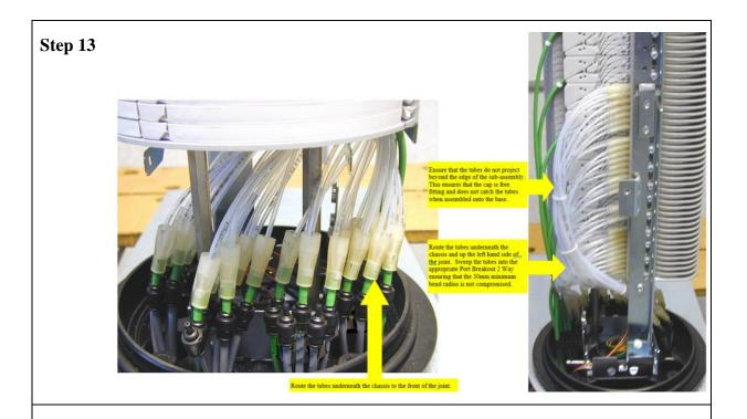
• Route the Transport Tubes (3) under the joint chassis to the front of the joint. At the front of the joint, route the tubes up the left-hand side and sweep them into the appropriate Port Breakout 2 Way ensuring that the 30mm minimum bend radius is not compromised. Ensure that the tubes do not project past the left-hand edge of the sub-assembly. This ensures that the cap is free fitting and does not catch the tubes when assembled to the base.
