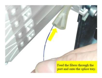
• Feed the fibres through the inner port of the Port Breakout 2 Way (2) and onto the Splice Tray.
