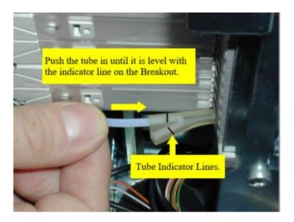
• Plug the tube into the entry port of the Port Breakout 2 Way (2) and push until the tube is correctly located down to the indication line.
