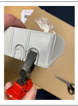
• Begin by removing the breakout, using plyers, apply light force and pull.
