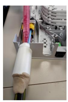
• After ensuring everything is in place, use compound 16 then insert the resin 10b into the funnel as shown.
