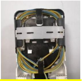
A single loop should be remaining after several coils have been installed.
