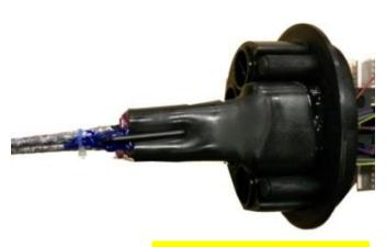
Complete the heat shrinking of the oval sleeve
