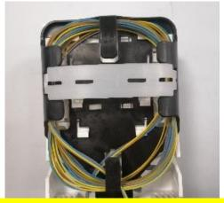
A single loop should be remaining after several coils have been installed.
