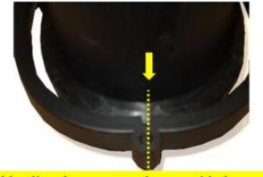
Roughly align the arrow on the cap with the centre of the clamp post to ease installation of the clamp
