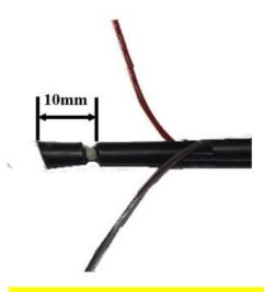
Cut polyethylene coating back 10mm
