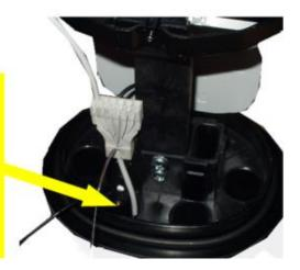
• Slide the tube over the first fibre/s and locate the end into the rear left-hand slot of the 2x12 Manifold (4). Push the tube down until the stop position is reached.
