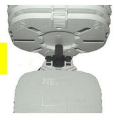
• Insert the tray retention tool the opposite way up from before, into the slot in the joint spine, directly below tray 2. Push until it locks.
