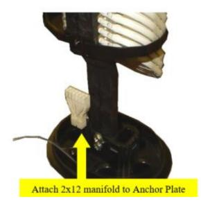
• Attach the 2x12 Manifold (4) to the Cable Anchor Plate (3) and press firmly into place.
