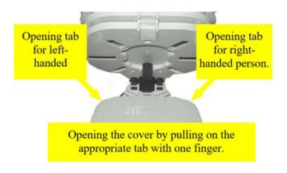
• Open the splice tray cover by pulling on either the left- or right-hand opening tabs as shown above.
