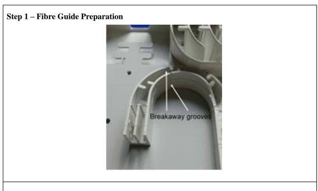
• The fibre guide supplied with the MDU internal splitter node incorporates breakaway grooves. This enables the left-hand side of the guide to be snapped off enabling installation of loop kit.
