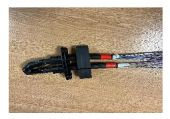
• Assemble 2 parts of external plate to cable butt end.
