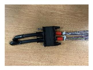
• Insert screws into assembly and lightly screw together in place.
