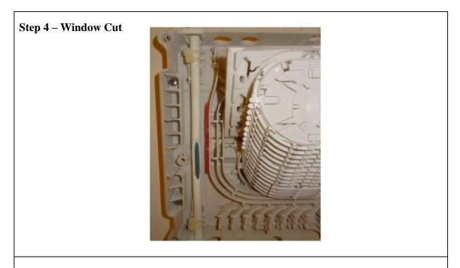
• Using the Pullback Cable Window Cutting Tool, remove the window, starting at the mark and going down towards the bottom of the box. The overall window cut is 70mm long.
