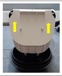
Push the tabs upwards to release the splice tray cover
