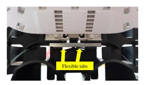
• Ensure the splitter is pushed right to the back of the slot and secured in place with the flexible tabs.
