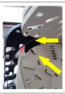
• Once the correct tray is reached, route the fibres into the track at the back of the manifold.
