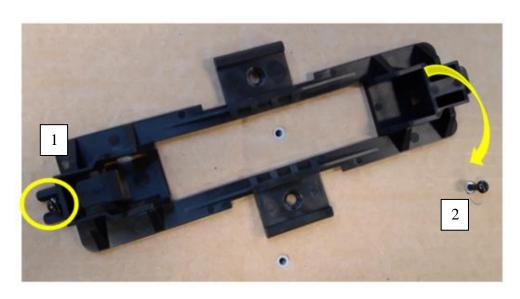
• Slide the horizontal groove into position first, then rotate the bracket about the screw to fit the vertical groove over the second screw.
