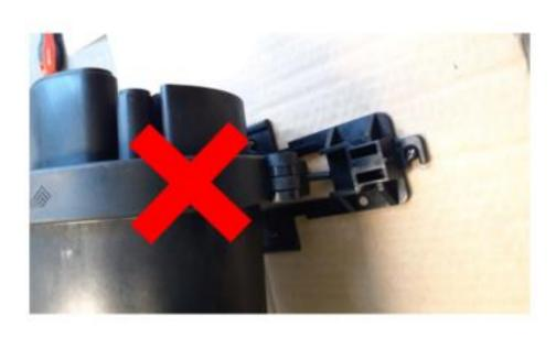
**NOTE**: Clamp on joint should be removed and rotated if installed upside down.
