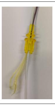
• Splay aramid evenly over the inner body and slide over outer body and click into position.
