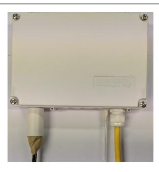
Fit cover and tighten the 4 retaining screws.
