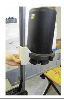
• To lower the joint press the plunger and lower the joint until it reaches the bottom locking position.
