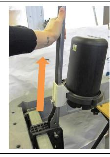
• Whilst holding securely, lift the joint and Mobra Arm vertically to release the locking mechanism.
