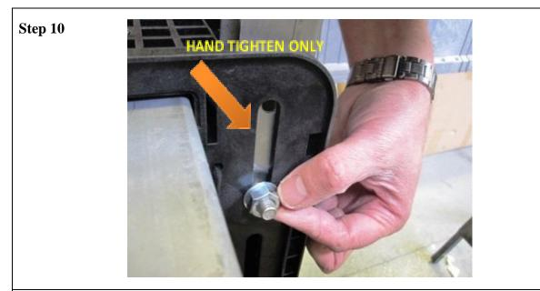
• Fit M10 washer to the other side and fit the M10 nut.
