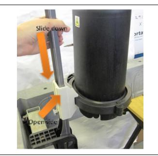
• Lower the MOBRA Arm into the MOBRA Knuckle so the arm fully inserts.
