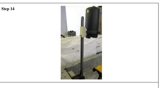
• To raise the joint press the plunger and lift the joint until it reaches the top locking position.
