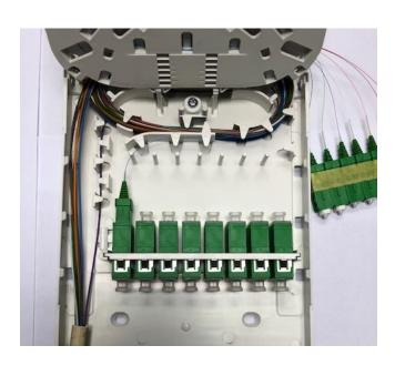
• Connect the SC connectors to the SC couplers by removing the protective caps.
