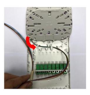
• Start to store the Mid-span from the top end of the cable and route as seen in the above picture.
