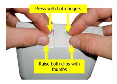
• To open the lid, press the clips on the top of the lid with both index fingers while lifting the thumbs off the base.
