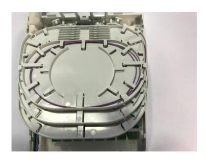
• Loop each fibre module in the splice tray fibre storage area.
