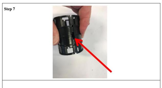
• Clip the 2 parts of the gland removal tool together by pushing the tabs into the other half.
