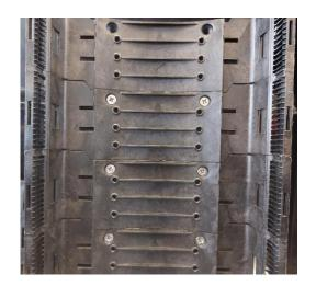
TO INSTALL AN ADDITIONAL SOSA/SASA UNIT FIRST IDENTIFY THE GROOVES IN WHICH THE NEW UNIT SLOTS INTO.
