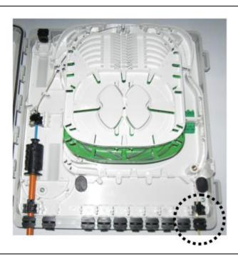
• Use the Cable Clips as described in the dedicated section. Install the cable clips with the right diameter on the Customer Cable in circled positions.
