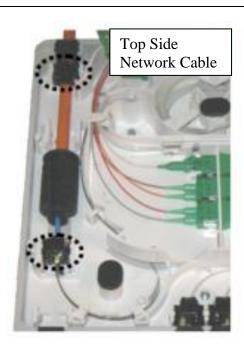
• If Network Cables comes from Top Side, then install cable clips with the right diameter on the tube and on the cable in circled positions.
