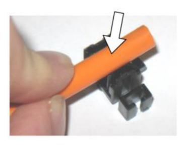
• Push the cable/tube into the cable clip.
