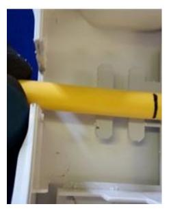
• Place the input side of the COF 201 cable into the bottom port slot and mark the sheath just above the cable retention bracket.
