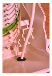
**Note:** The Customer Premise Cable ports consists of 3 rows of 12 ports and count from the back row LEFT TO RIGHT when viewed from the top.
