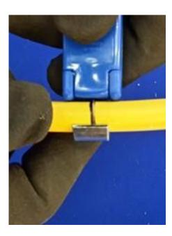
• Circumferentially cut the COF 201 sheathing at the two marks using a stripper cable sheath 7 item code 126853.
