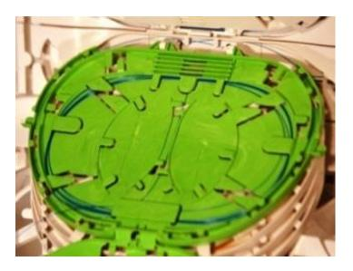
**Note:** The Splitter device input fibres are pre-installed into the (green) device tray such that the nominated working fibre (blue) is in TR AY 1.
