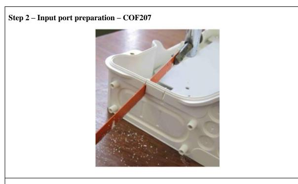
• Saw along moulded guides and snap off remaining material to form a cable access slot at top and bottom of closure left side.
