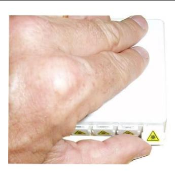
• The shutters on the adapters can then be rotated open to plug in SC patch cords when required.
