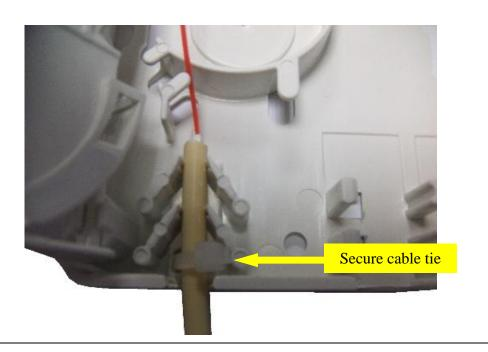
• Push the cable down into the grips and secure the cable tie.
