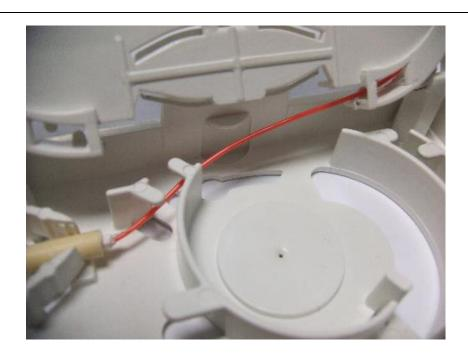
• Route the fibre underneath the tabs as shown and into the entry port of the splice tray.
