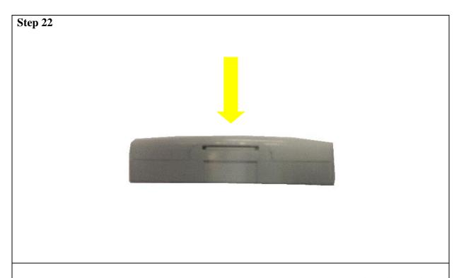
• Replace the cover by pressing onto the base until it clicks into place.
