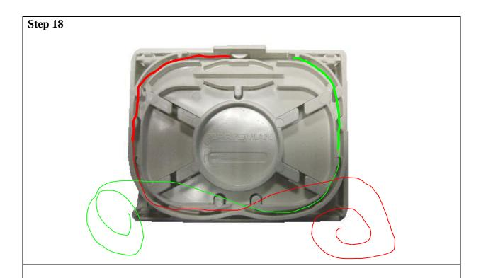
• Uncoil the pigtail and cable fibres from the tray, back to the point shown above.
