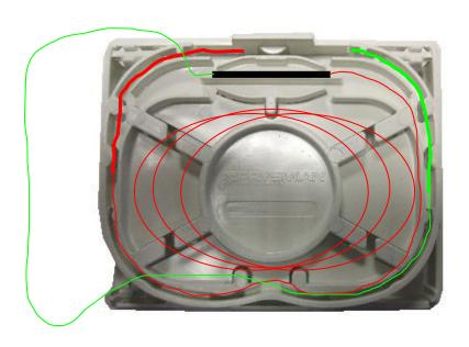
• Take the cable fibre loop and coil the fibre around the splice tray and the track to the splice protector bay as shown.
