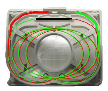
• Take the pigtail fibre loop and coil the fibre around the splice tray and the track to the splice protector bay as shown.
