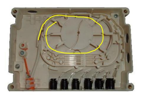
• Route the fibres around the track into the central storage area of the splice tray, and coil beneath the tabs to store for later use.
