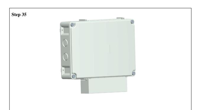
Replace the main cover and secure by tightening the four screws.
