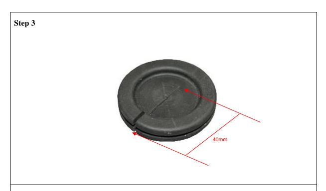
Using a sharp a sharp knife or a pair of scissors cut a slot in the cable entry bung approximately 40mm long as shown above for inserting the cable.
