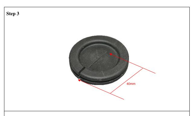
Using a sharp a sharp knife or a pair of scissors cut a slot in the cable entry bung approximately 40mm long as shown above for inserting the cable.
