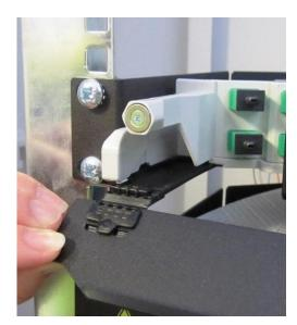
• Gently place your fingers on the cover and pull down to release the magnetic grip and leave to hang freely exposing the patch cord adapters.
